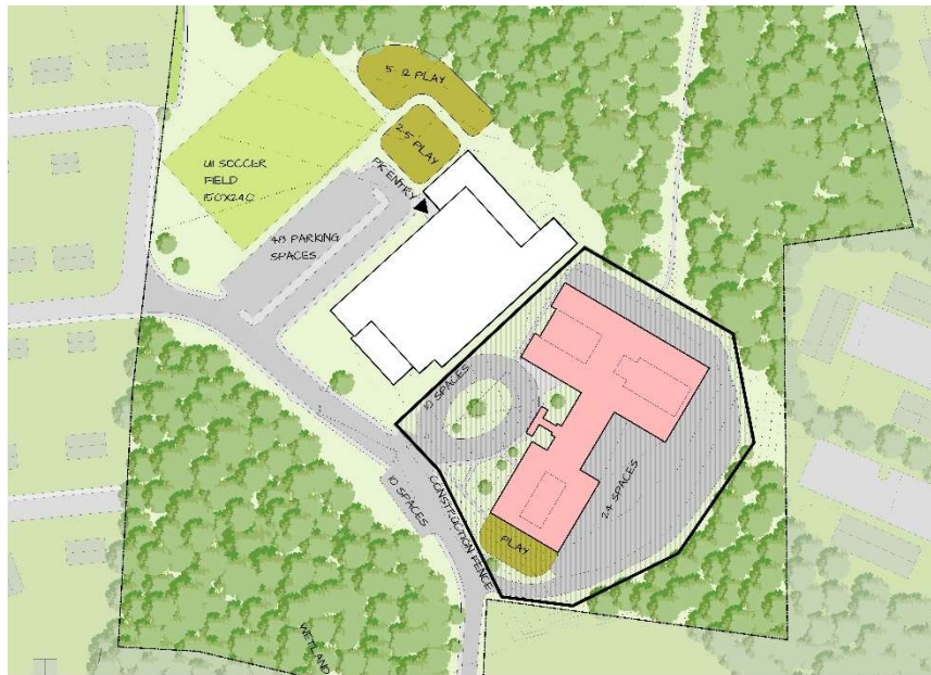
Phasing Diagram for Option 3: When the new building is complete and in use, demolition of the existing building begins.
